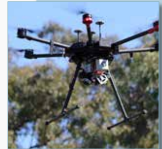
DJI Matrice M600 equipped with RIEGL miniVUX-SYS using RIEGL Integration Kit 600
